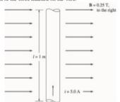
SOLUTION The force on this wire can be calculated from the equation
