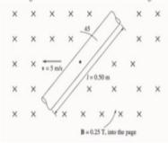
$S_{OLUTION}$  The induced voltage on this wire can be calculated from the equation shown below. The voltage on the wire is positive downward because the vector quantity  $\mathbf{v} \times \mathbf{B}$  points downward.
