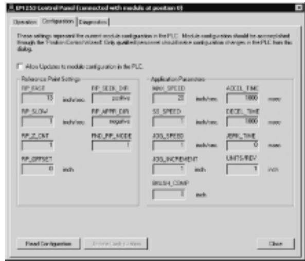
Figure 9-20 Configuration Tab of the EM 253 Control Panel
