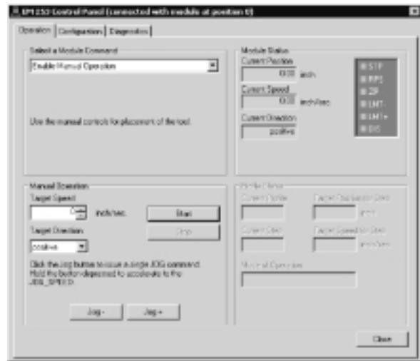
Figure 9-19 Operation Tab of the EM 253 Control Panel
